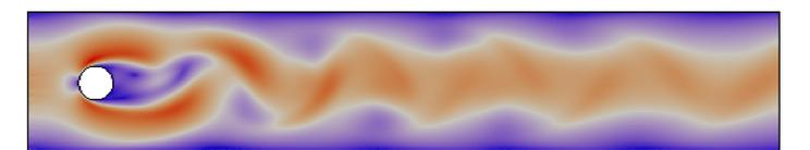
Figure 7: Velocity magnitude plot with entropy conservative scheme and viscous fluxes
