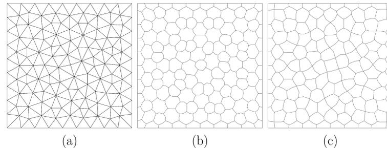
Figure 1: Unstructured meshes (a) Primary (b) Median dual (c) Voronoi dual
