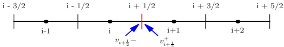
$$\begin{aligned}v_{i+\frac{1}{2}}^- &= v_i + \frac{1}{2} \text{minmod}(\Delta v_{i+\frac{1}{2}}, \Delta v_{i-\frac{1}{2}}) \\v_{i+\frac{1}{2}}^+ &= v_{i+1} - \frac{1}{2} \text{minmod}(\Delta v_{i+\frac{3}{2}}, \Delta v_{i+\frac{1}{2}})\end{aligned}$$
