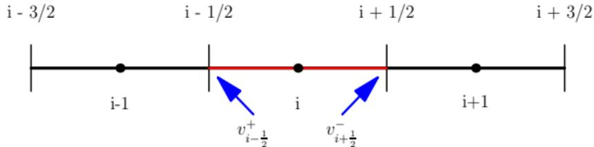
$$\text{sign}(v_{i+\frac{1}{2}}^- - v_{i-\frac{1}{2}}^+) = \underbrace{\text{sign}(\Delta v_{i+\frac{1}{2}})}_{\text{if true}} = \underbrace{\text{sign}(\Delta v_{i-\frac{1}{2}})}_{}$$
